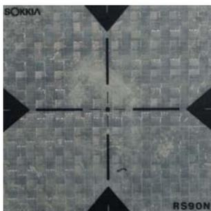
**Figure 4.2.1 Reflector sheet**
