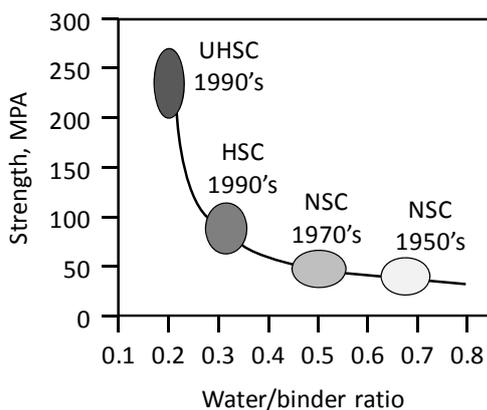
Figure 4 Development of concrete strength over time (Bentur, 2002)
