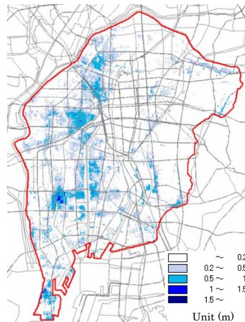
Figure 3.4 Maximum inundation water depths (CASE II)
