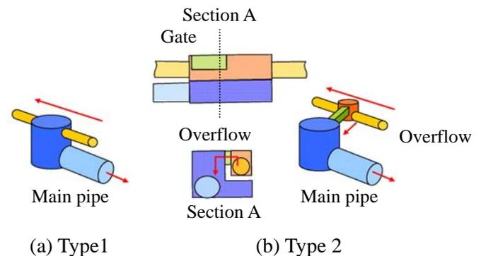
Figure 3.1 Manhole-sewer structure on water transport
