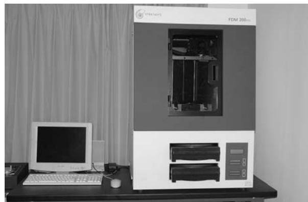
Figure 2 Rapid prototyping Facility (FDM 200)
