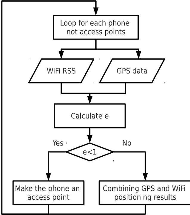
Figure 6: The process of the adjusting algorithm.
