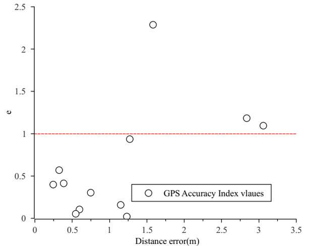
Figure 2: Using RSS serial and GPS distance between two smart phones to calculate the GPS accuracy index.
