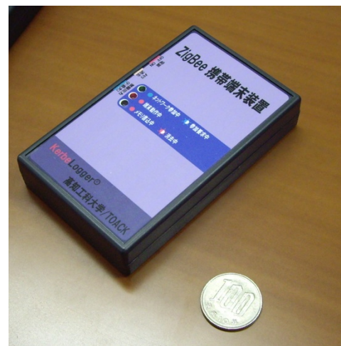
Figure 8 New devices which integrated ZigBee wireless communication system and acceleration sensor
