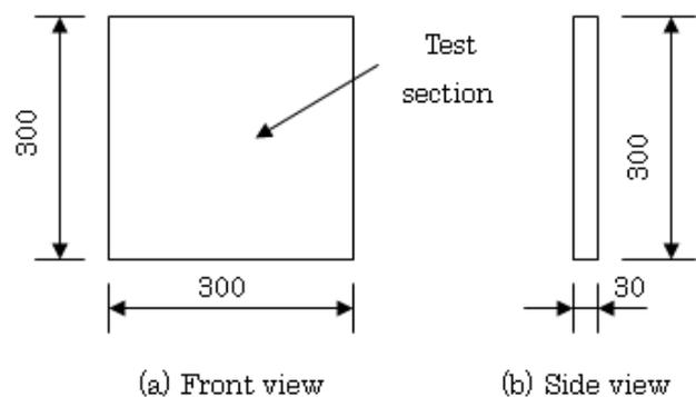
Fig. 4 Concrete plate specimen "impact flow" (mm)
