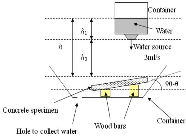
Fig. 5 Setting of concrete plate specimen “impact flow”
