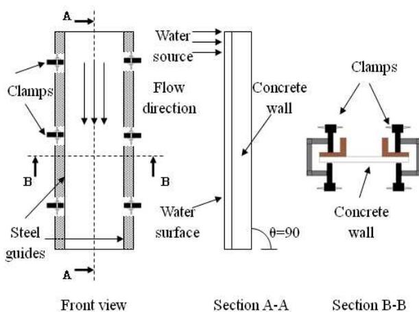
Fig. 2 Setting of concrete plate specimen "film flow"
