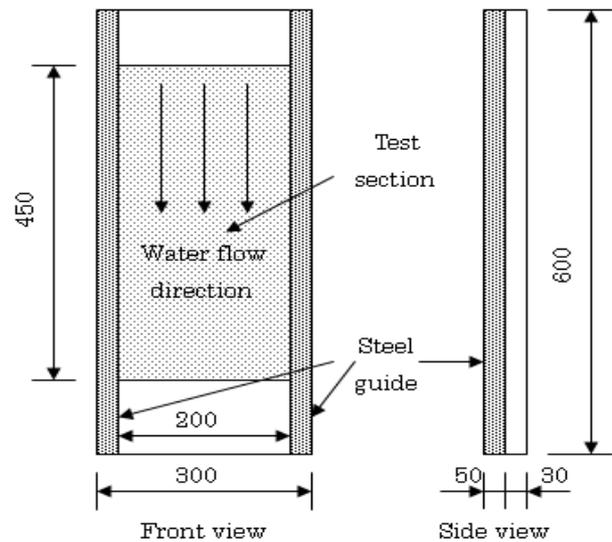
Fig. 1 Concrete plate specimen "film flow" (mm)
