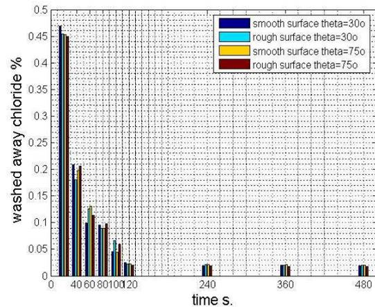
Fig. 10 Washed away chloride% “dry and impact water”
