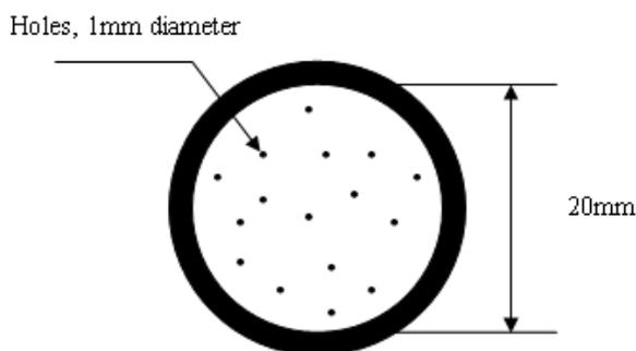
Fig. 6 Outlet of water flow
