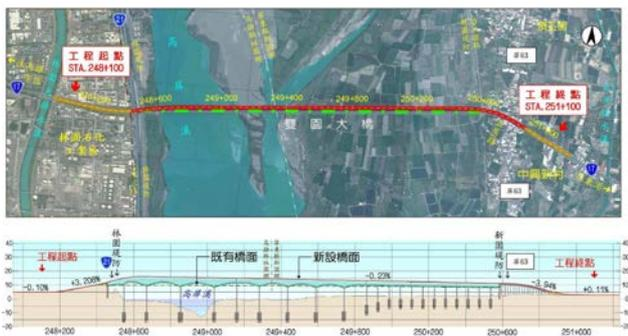
Figure 2 Option one layout, full offset from old bridge
