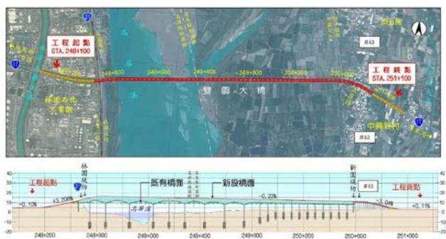
Figure 3 Option two layout, partial offset from old bridge
