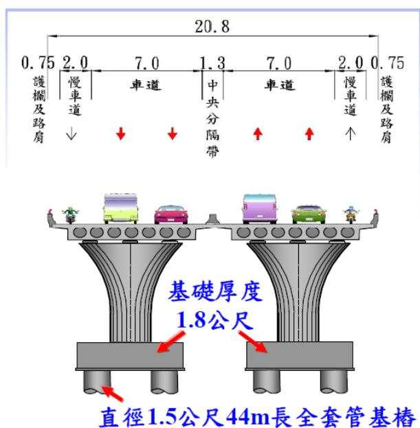
Figure 5 Cross section of approach bridge
