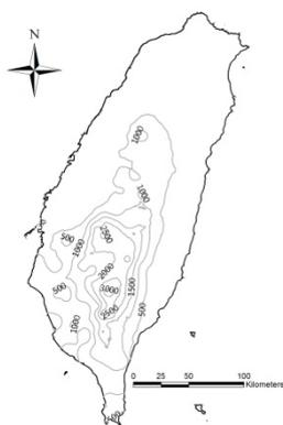
Fig. 1 Isohyets of Taiwan during Typhoon Morakot. Isohyets are in mm depth of total rainfall.
