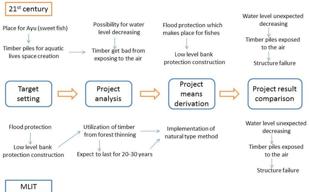
**Figure 12** Comparing mental models on failure revetment work
