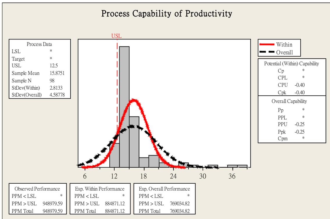
**Figure 4.3** Process Capability of Column before improvement
