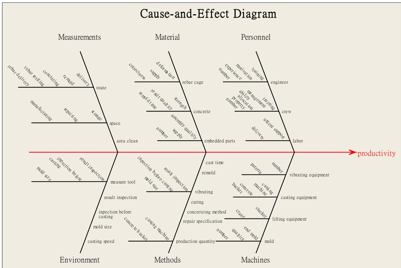
Figure 4.2 Cause-and- Effect Diagram of affecting productivity
