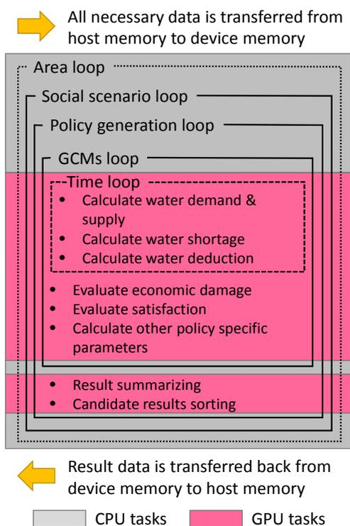
Figure 8. Tasks distribution between CPU and GPU
