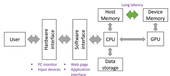
Figure 7. Data flow among user, CPU, and GPU
