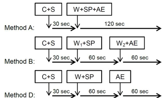
Fig. 7: Three types of mixing method for mortar;
