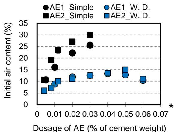
Fig. 5: Effect of water-dividing mixing method (W. D.) on initial air content (\*dosage of AE  $\times$  4 in case of AE2)
