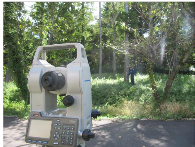
Figure 2.8 State of the tree height measurement using a TS and prism
