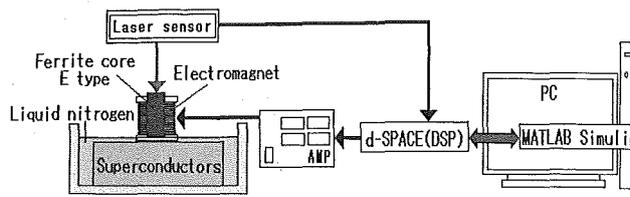
Fig. 7 Experimental setup for levitation
