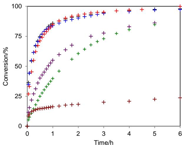
**Fig. 1** Time/conversion curves for **3** in different solvents. Acetonitrile (+), THF (+), benzene (+), chloroform (+), methanol (+), and acetone (+). The reaction conducted at 30 °C using a 0.06 M solution.
