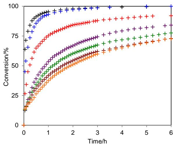
**Fig. 2** Time/conversion curves for **3** under various concentrations. 0.24 (+), 0.12 (+), 0.06 (+), 0.03 (+), 0.025 (+), 0.02 (+), and 0.015 (+) M. The reaction conducted at 30 °C using benzene-*d*<sub>6</sub> as a solvent.
