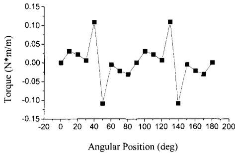
Fig. 10. Torque when control current arrangement for vertical force is applied
