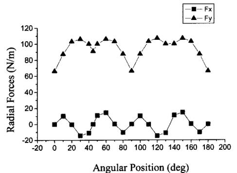
Fig. 9. Radial forces about rotor angular position
