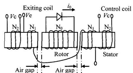
Fig. 2. Schematic of stator and rectified rotor
