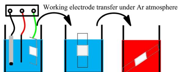
**Figure 1.** Schematic representation of the immobilization procedure.
