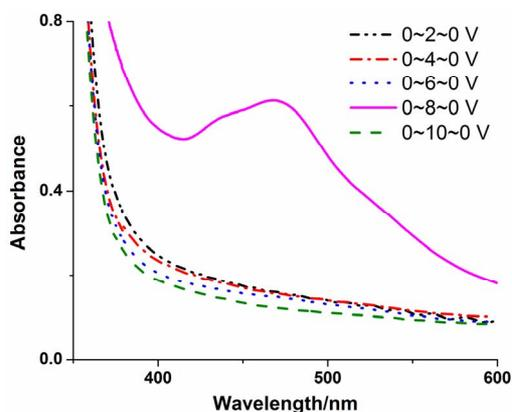
Figure 3. Uv-vis spectra of the resultant  $\text{TiO}_2/\text{FTO}$  electrodes.
