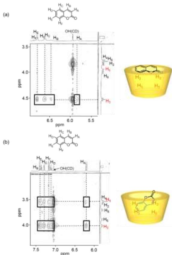
**Figure 2.** Partial NOESY spectra and proposed structure of the 1 : 1 complexes between TBDMS- $\beta$ -CD ( $1.0 \times 10^{-3}$  M) and coumarin ( $1.6 \times 10^{-2}$  M) (a) in benzene- $d_6$  and (b) in cyclohexane- $d_{12}$ .
