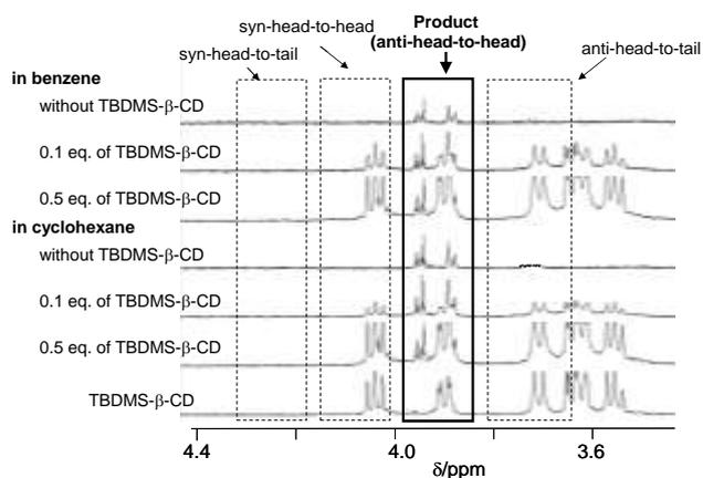
**Figure 3.** Partial <sup>1</sup>H NMR spectra of the dimers (the cyclobutane proton region) obtained upon irradiation of coumarin at 10 °C for 24 h in benzene and cyclohexane in the absence and presence of TBDMS- $\beta$ -CD (solvent : CDCl<sub>3</sub>).
