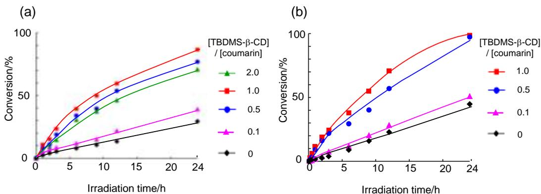
**Figure 4.** Time course of the photodimerization of coumarin (0.027 mmol) in the presence of different amounts of TBDMS- $\beta$ -CD in (a) benzene and (b) cyclohexane (10 mL) at 10 °C.
