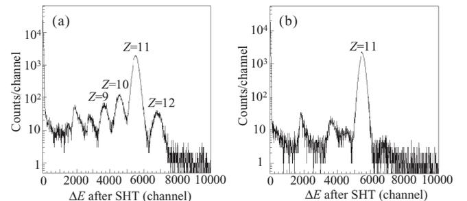
FIG. 3. (a) Typical  $\Delta E$  spectrum for  $^{32}\text{Na}$  measured by a stack of Si detectors located after the solid hydrogen target (SHT). Peaks for  $Z = 9, 10, 11$ , and  $12$  are clearly seen. (b) Same spectrum, but without SHT.
