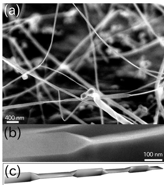
**Figure 1** | (a) SEM image of chains of carbon nanotetrahedra/nanoribbons. (b) Enlarged SEM image of a carbon nanotetrahedron. (c) Three-dimensional schematic model of a chain of carbon nanotetrahedra/nanoribbons.
