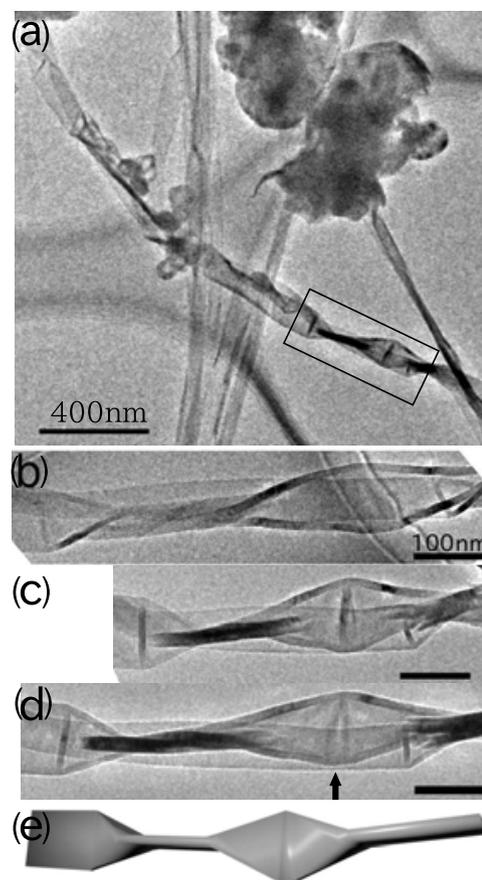
**Figure 3** | (a) TEM image of a nanoribbon with two adjoining nanotetrahedra. (b)–(d) Enlarged images viewed along different directions. (e) Schematic 3D model of the nanoribbon with adjoining nanotetrahedra.
