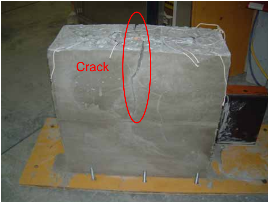
Photo-6.3 Paste specimen R1-E/(C+E) =6.5% (after mold removed)
