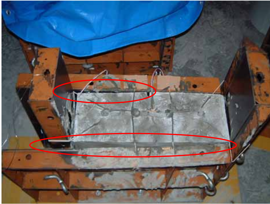
Photo-6.1 Paste specimen R1-E/(C+E) = 6.5% (before mold removed)
