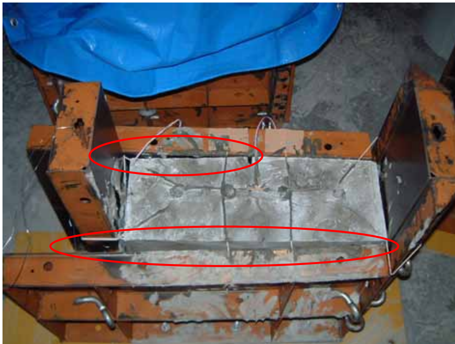
Photo-6.1 Paste specimen R1-E/(C+E) = 6.5% (before mold removed)
