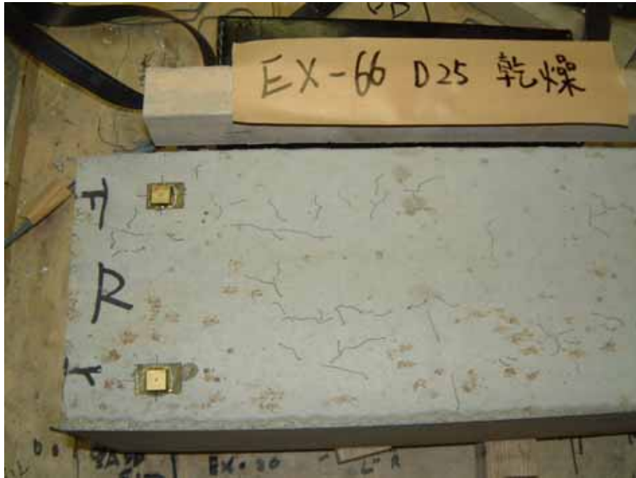
Photo-3.1 Crack occurred on the surface of drying-curing specimen due over-expansion (EX66)
