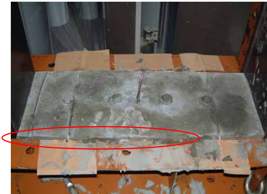
Photo-6.2 Paste specimen R2-E/(C+E) = 6.5% (before mold removed)
