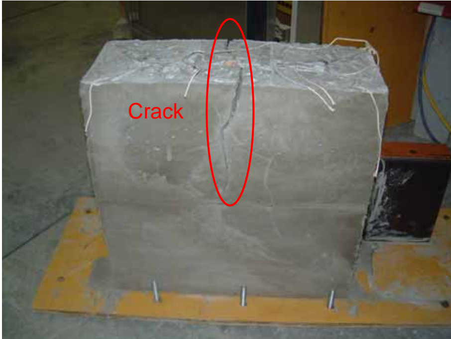
Photo-6.3 Paste specimen R1-E/(C+E) =6.5% (after mold removed)
