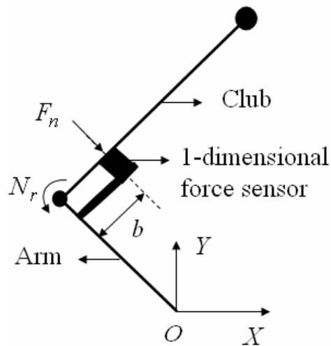
Figure 5-8 Obtainment of the reaction torque  $N_r$
