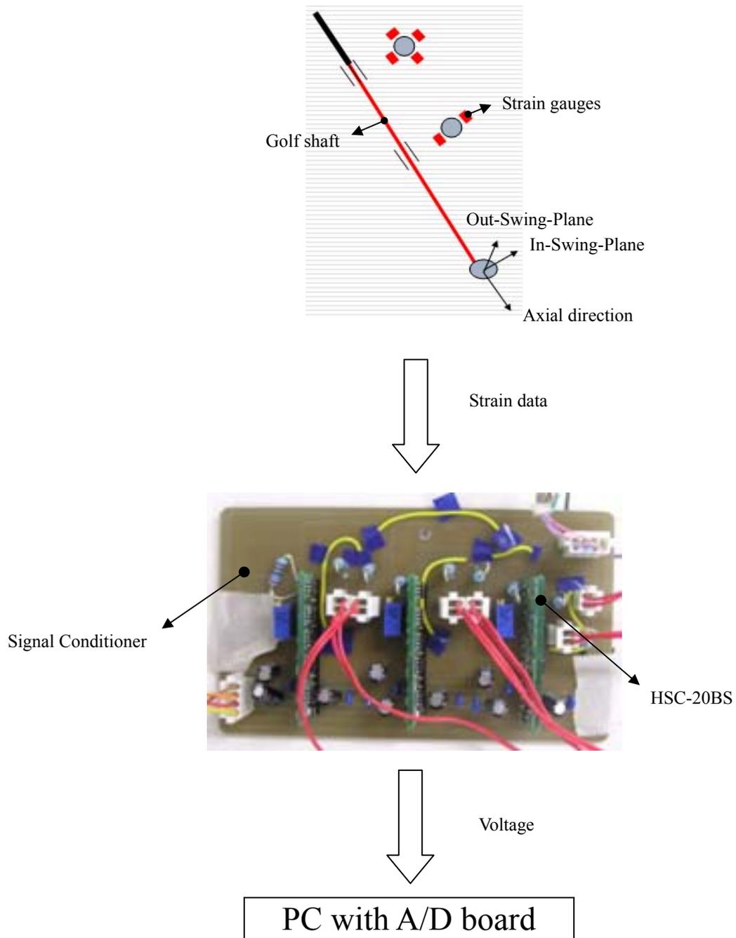
Figure 3-4 Configuration of strain data collection system
