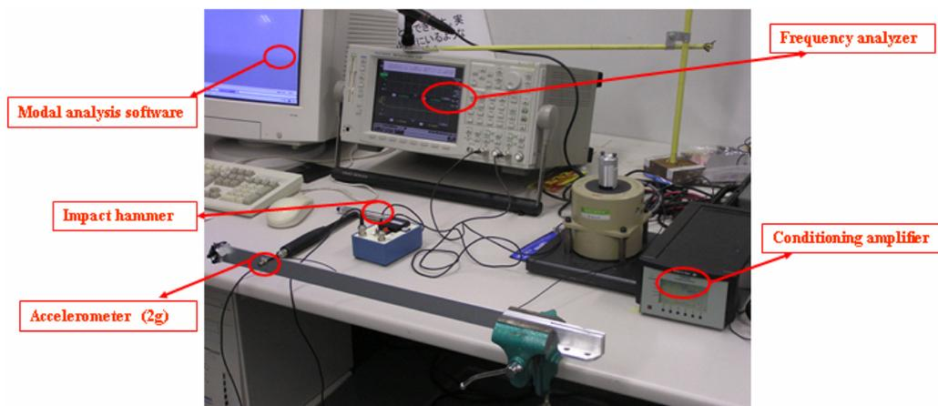
Figure 5-4 Configuration of the modal analysis system
