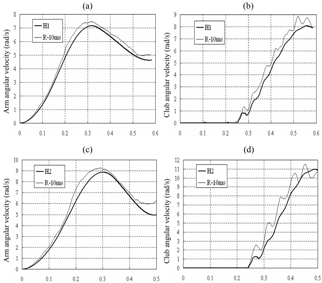
Figure 5-15 Comparison of arm and club angular velocities for the robot and different-arm-mass golfers using the 10 ms sampling control period
