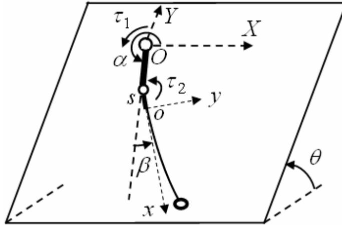
Figure 3-1 Dynamic model of golf swing. The torque  $\tau_1$  is applied at the shoulder joint  $O$  to drive the swing; the torque  $\tau_2$  is employed at the wrist joint  $s$  to hold golf club. The rotational arm angle is  $\alpha$  and the club angle is  $\beta$ .
