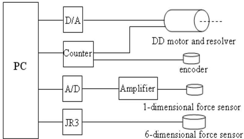
Figure 5-7 Schematic diagram of the experimental control system
