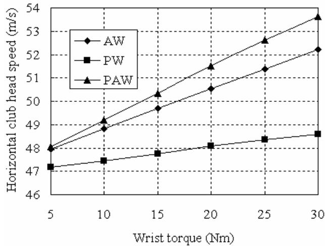
Figure 2-2 Maximal horizontal club head speed at impact by maximum criterion.
