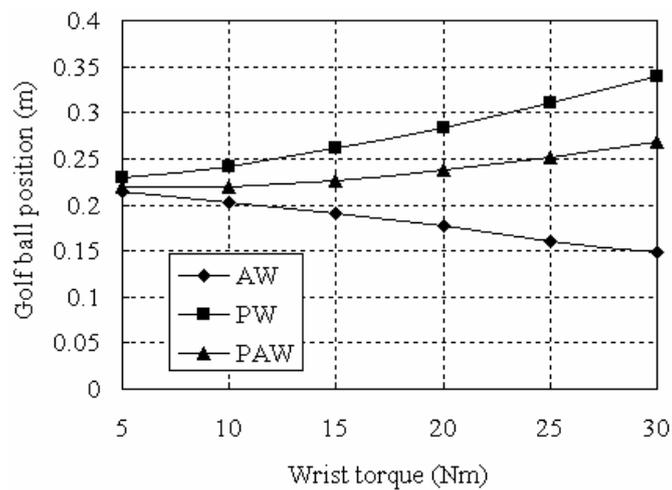
Figure 2-3 Optimum golf ball position by maximum criterion.
