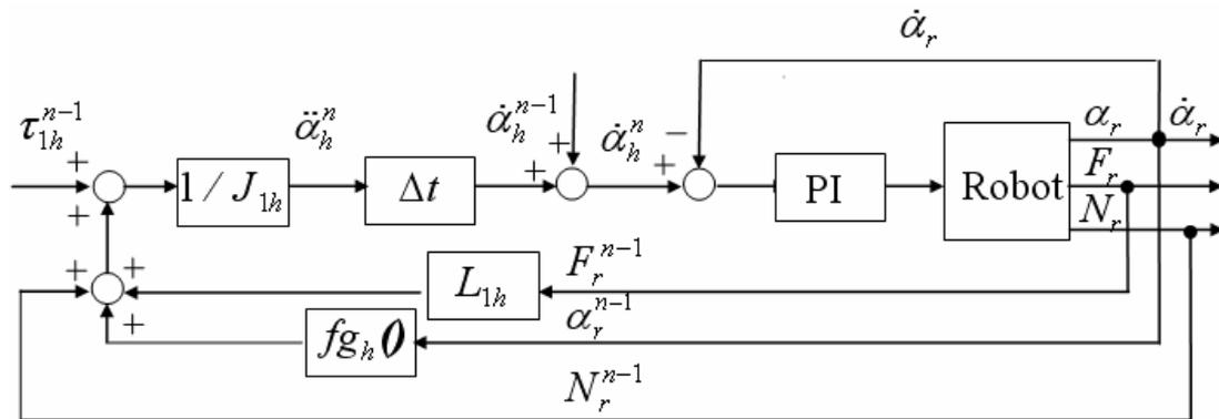
Figure 5-3 Configuration of the control system
