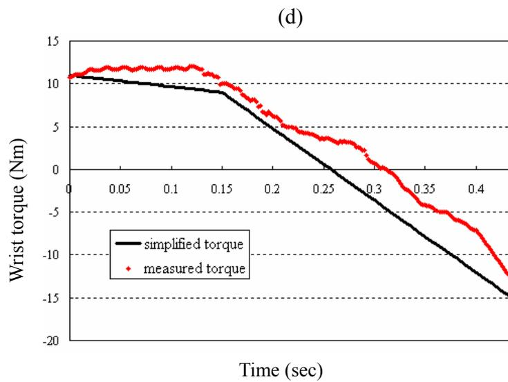
Figure 3-5 Measured and simplified torques for the shoulder and wrist joints. (a) shoulder torque for subject A; (b) wrist torque for subject A; (c) shoulder torque for subject B; (d) wrist torque for subject B;
