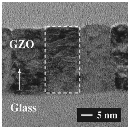
FIG. 2. Cross-sectional TEM image of the GZO film with a thickness of 30 nm. A single column is indicated by a broken line.
