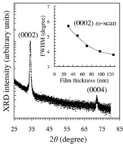
FIG. 1. Typical XRD  $\theta$ - $2\theta$  scan profile of the GZO film with a thickness of 30 nm. The diffraction intensity on the vertical axis is expressed in a logarithmic scale. The inset shows the full width at half maximum of (0002)  $\omega$ -scan rocking curve as a function of film thickness below 98 nm.
