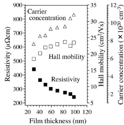
FIG. 3. Resistivity, carrier concentration, and Hall mobility of GZO films as a function of film thickness in the range from 30 to 98 nm.
