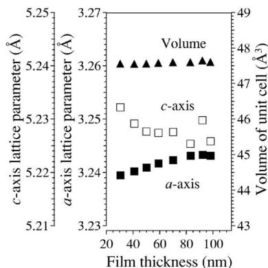
FIG. 4. Lattice parameters of  $a$  and  $c$  axes in GZO films as a function of film thickness below 98 nm. These parameters are determined by the analysis of in-plane and out-of-plane XRD peak profiles. The volume of the crystallographic unit cell, calculated with the lattice parameters, is also shown.
