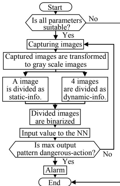
Fig. 5: The procedure of the awakening behavior detection
