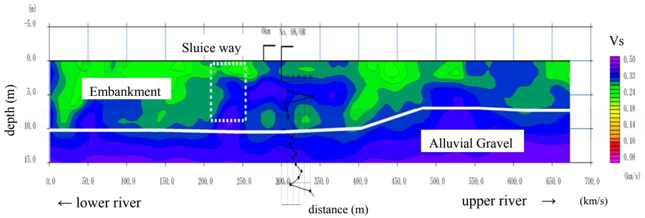
Fig. 7 S-wave velocity contour
