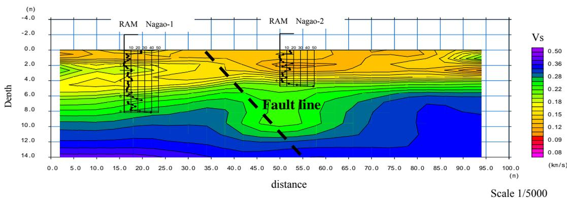
Fig. 4 S-wave velocity contour at Tanaka site
