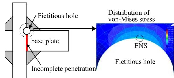
Fig.5 Distribution of von-Mises stress around fictitious hole
