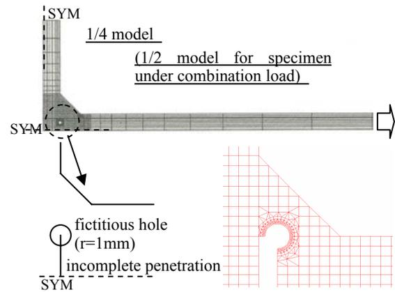
Fig.4 FE model for calculation of ENS
