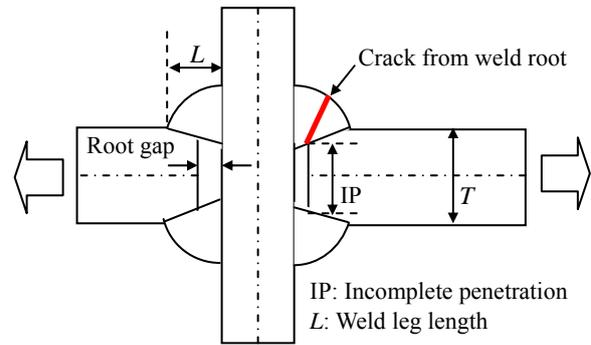
Fig.6 Crack from weld root of load carrying cruciform welded joint
