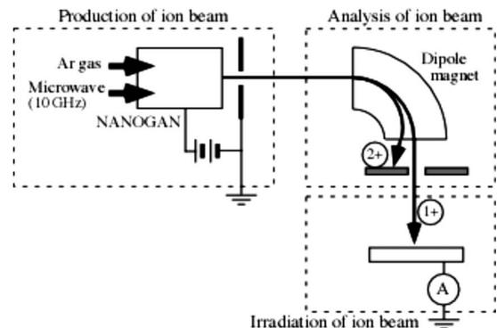
FIG. 2. Schematic picture of the irradiation equipment for  $\text{Ar}^{1+}$  ion beam.
