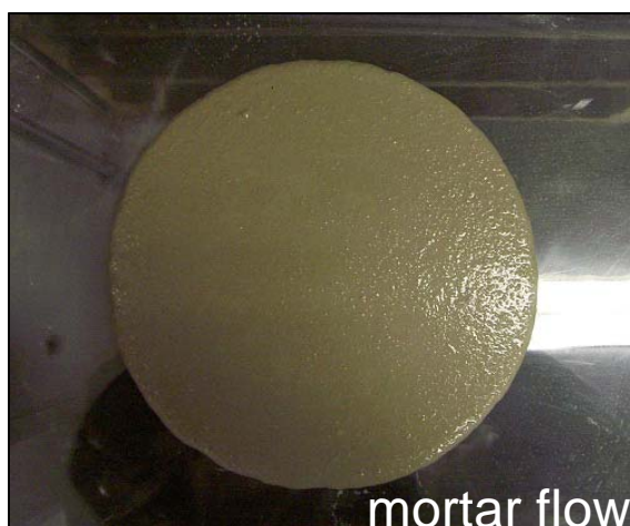
Fig. 8 Flow of self-compacting mortar of around 300 mm
