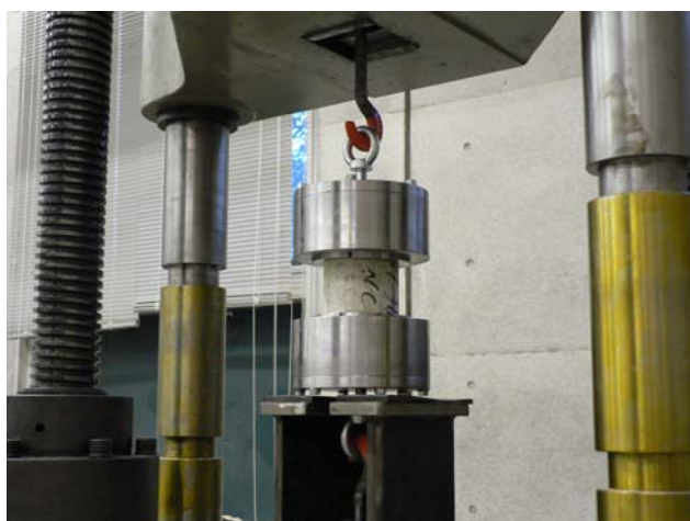
Fig. 11 Chuck type of tensile testing apparatus
