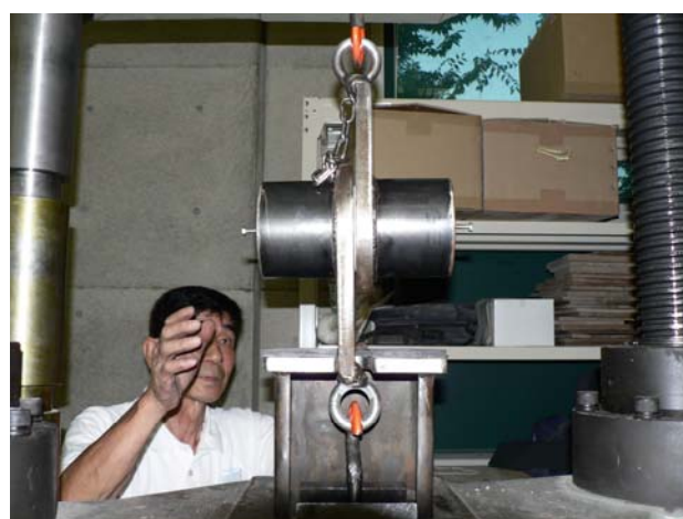
Fig. 13 Direct pure shearing testing apparatus: not by compression but by tension
