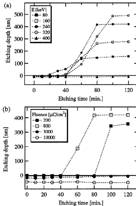
FIG. 3. Etching depth of Si as a function of the etching time.  $\text{Ar}^{4+}$  ions were irradiated onto Si. (a) The beam energy  $E$  was varied over the range of 80–400 keV. The fluence of Ar ions was  $800 \mu\text{C}/\text{cm}^2$ . (b) The fluence of Ar ions was varied over the range of 200–10 000  $\mu\text{C}/\text{cm}^2$ . The beam energy was 240 keV.
