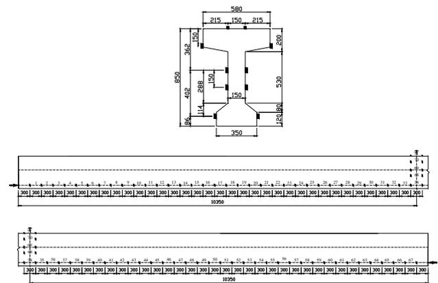
Fig.11 Position of gauge plug and measured camber
