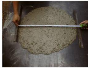
Slump flow test
