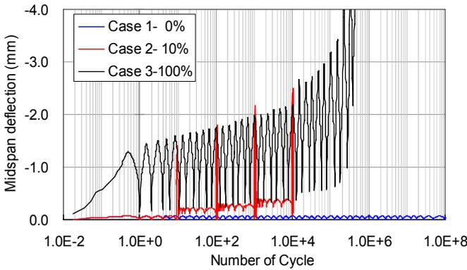
Figure 3.14 Mid-span deflections in comparison with heavy traffic.
