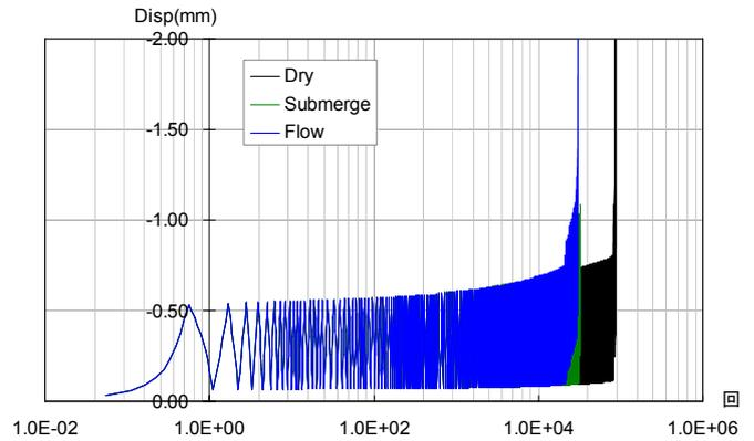
Figure 4.2 Mid-span deflections in progress under pulsating load
