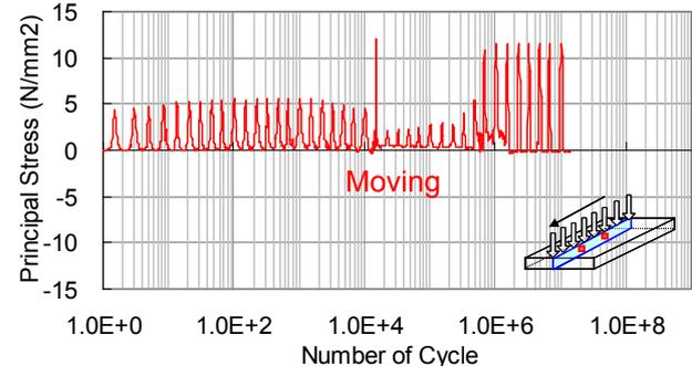
Figure 3.5 Principal stresses at the referential finite element concerned
