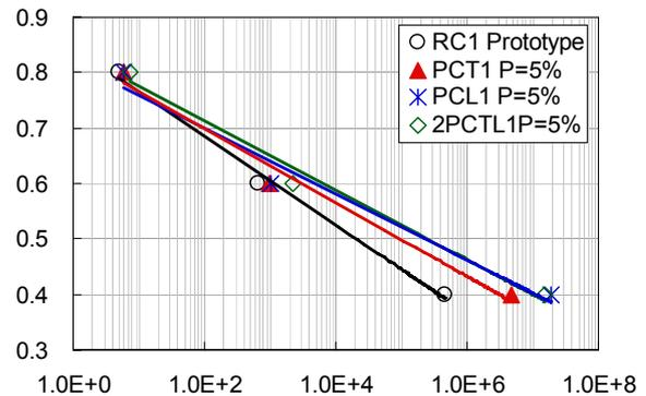
Figure 3.11 Normalized S-N diagrams regarding the pre-stressing directions
