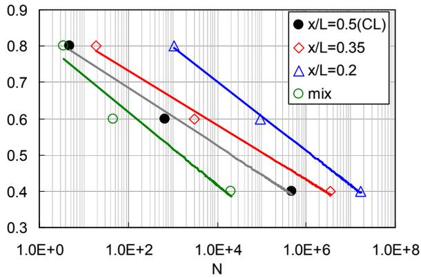
Figure 3.12 Normalized S-N diagrams for offset loading effect
