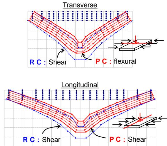
Figure 3.9 Cross section at the maximum load
