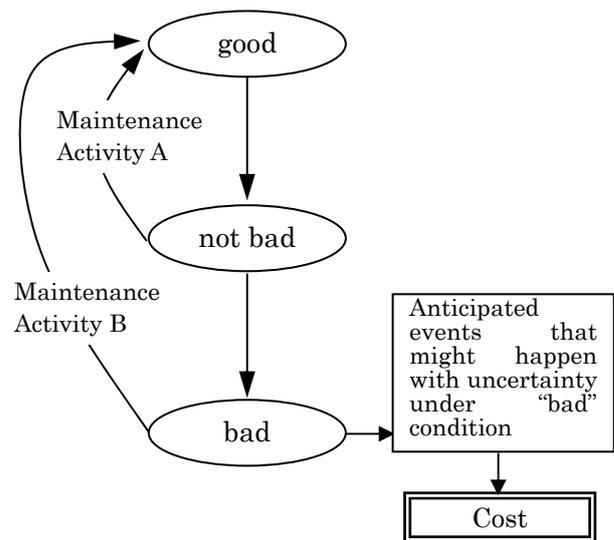
Fig.12 Modeling of consequent events in Markov deterioration
