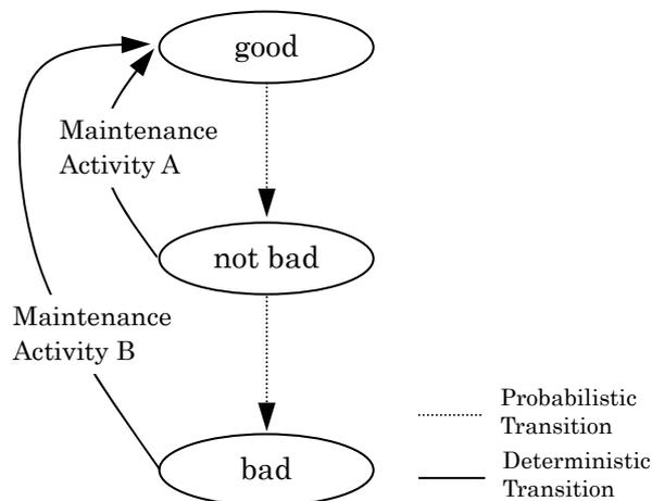
Fig.10 Modeling of maintenance in Markov deterioration model
