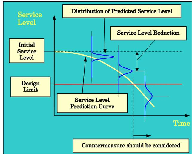
Fig.2 Behavior of self-deteriorating structures
