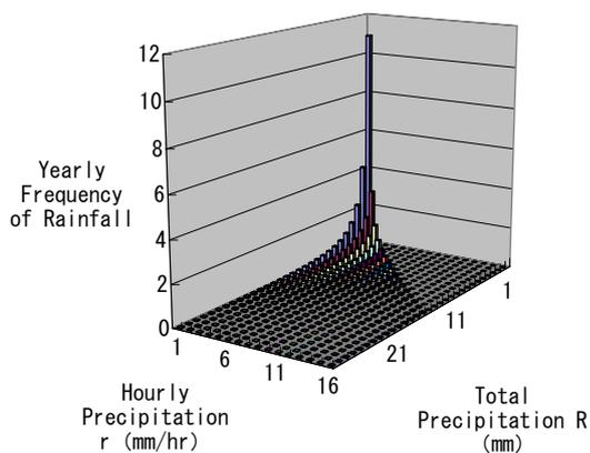
Fig.9 An example of two-dimensional hazard curve
