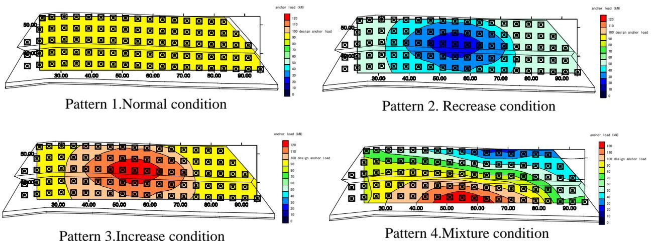
Figure 1. Distribution pattern of anchor load
