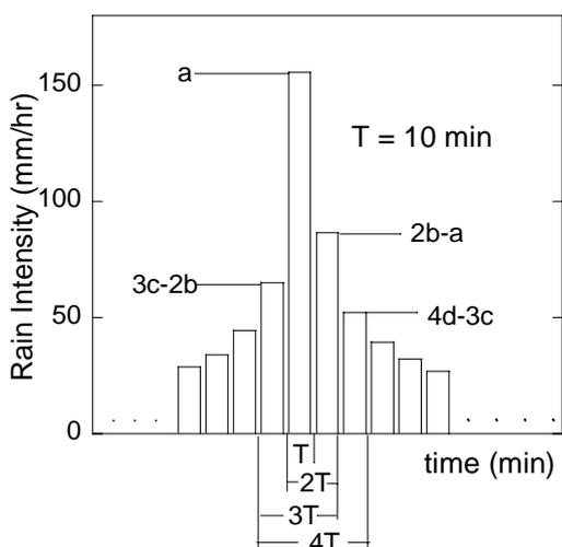
Fig.3(b) Hyetograph based on the IDF relationship and constructed by the alternating block method
