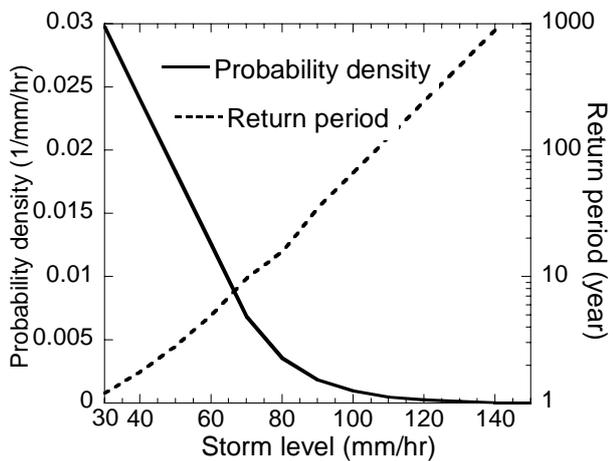
Fig.2 Storm probability curve. The curve relates storm level and its probability density. Storm level is also related to return period.
