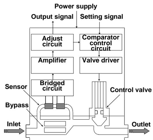
Fig. 1 Structure of a mass flow controller
