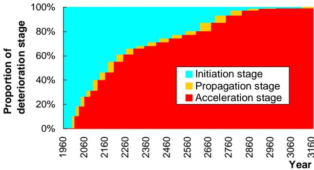
Figure 3.3 Time variation for proportion of deterioration stage
