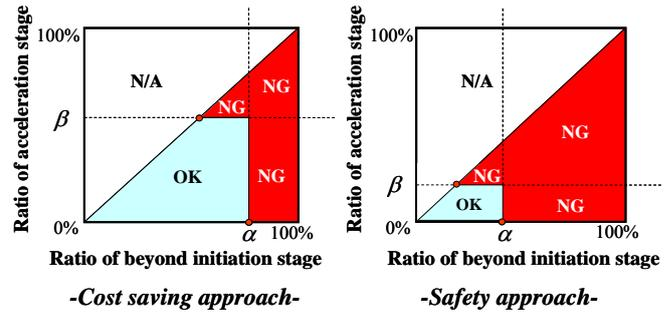
Figure 3.7 Definition of threshold  $\alpha$  and  $\beta$
