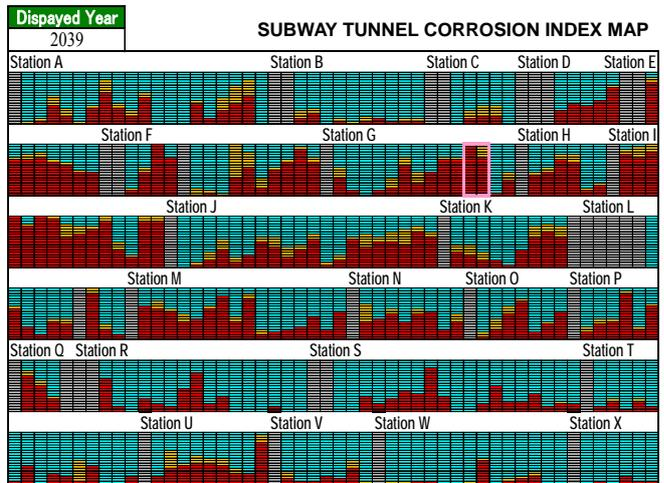
Figure 3.5 Corrosion index map 30 years later
