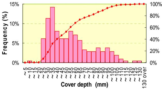
Figure 3.2 Measured cover depth in a control unit
