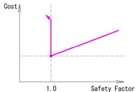
Fig. 2 Safety Factor of Construction VS Cost
