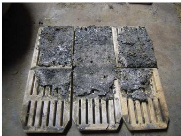
Picture 3. Clinker adhered to the ceramic rostile
