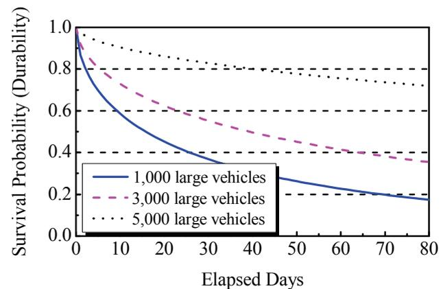
**Figure 6** Survival Probabilities of Patching Mixtures (Large vehicle traffic amount)
