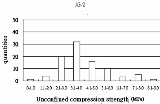
Fig. 7 qu distribution of in-situ cored samples in Japan
