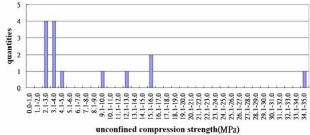
Fig. 5 Unconfined compression strengths of in-situ cored samples (Silty ground)
