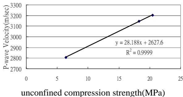
Fig. 8 qu versus P-wave velocity (in-situ cored samples)
