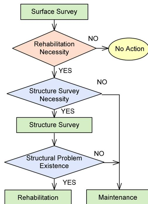
**Figure 1** Flow chart of evaluation and rehabilitation subsystems for airport pavement management
