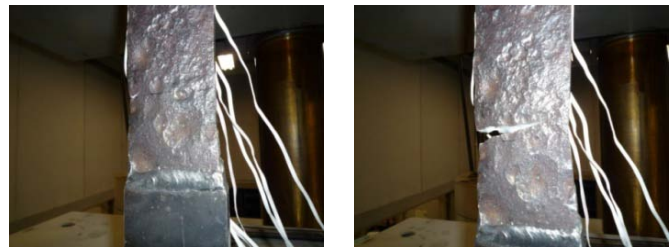
(a) Crack occurring (b) Crack progressing
