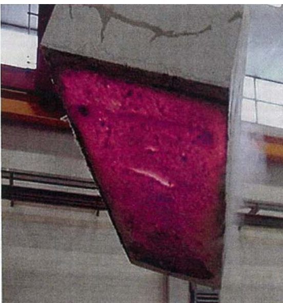
Figure 5.5 High temperature heated chemical fiber concrete specimen 7)
