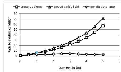
*Figure 10 Performance indicator ratio of each scenario of dam height.*
