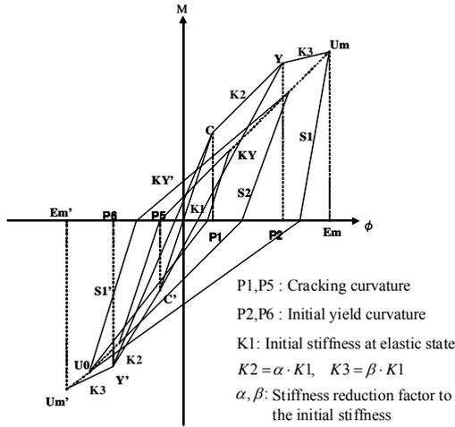
Fig.4 Trilinear rigidity hysteresis model for RC pier (Takeda model)
