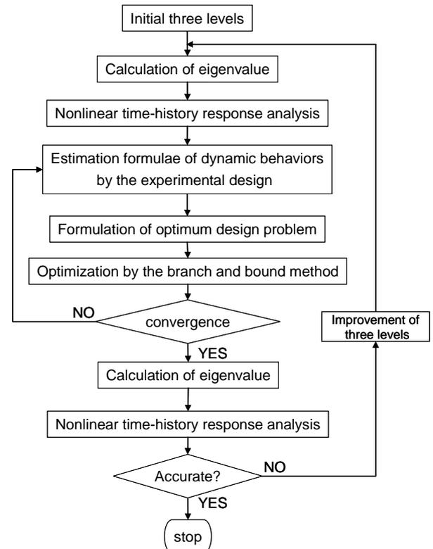
Fig.6 Macro-flow of the proposed optimum design method
