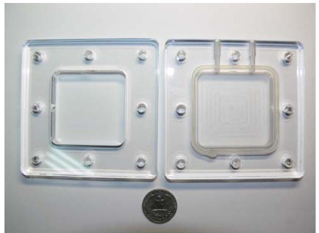
Photo 3.1.4 Completed two supporting plates
