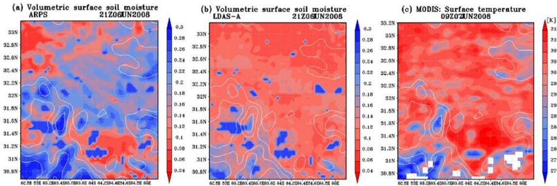
Fig. 4. Spatial distribution of simulated surface soil moisture contents ( $\text{m}^3/\text{m}^3$ ) at 0730 UTC on 6th June 2008; (a) ARPS (no-assimilation case), (b) LDAS-A, and (c) MODIS land surface temperature (K) at 0900UTC on 7th June 2008, contour lines depict topography.
