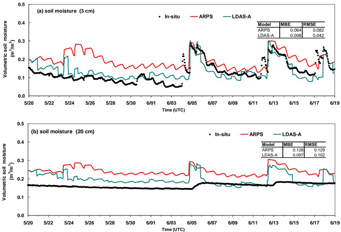
Fig. 5. Comparison of observed and simulated soil moisture content at the Gaize station from 20th May 2008 to 19th June 2008; (a) at 3 cm, (b) at 20 cm.
