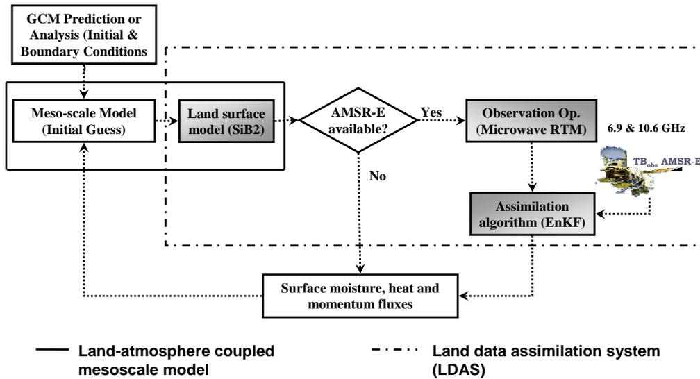
Fig. 1. Framework of the land data assimilation system coupled with an atmospheric model (LDAS-A)
