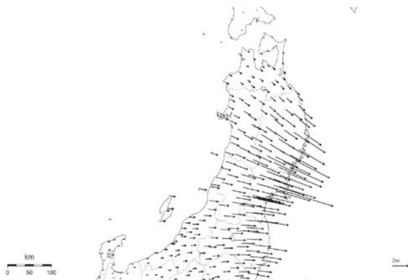
Figure 1.1 Measurement Results of displacement by GPS in Tohoku, JAPAN (© GSI)
