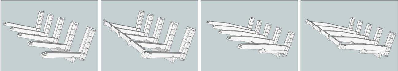
Figure 4.10 Reproduction of the bridge construction process (Soribashi)
